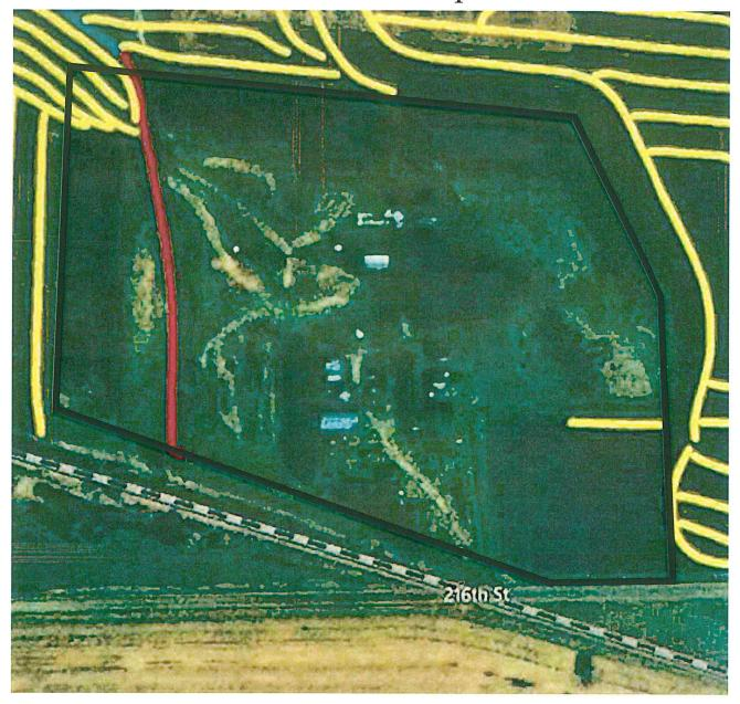
■ 10" Main Non Perferated Tile Line - Drainage Easement
